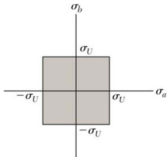
Brittle materials fail suddenly through in a tensile test. The failure condition is characterized
