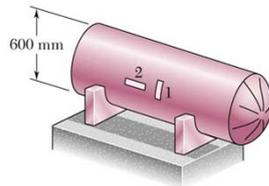
A cylindrical storage tank used to transport gas under pressure has an inner diameter of 600 mm and a wall thickness of 18 mm. Transverse and longitudinal strains are measured to  $255\mu$  and  $60\mu$  by two strain gages. Knowing that  $G = 77$  GPa, determine (a) the gage pressure inside the tank, and (b) the principal stresses and maximum shearing stress in the tank
