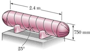
A compressed-air tank is supported by two cradles. The tank body is fabricated from a 10-mm steel plate welded along a helix that forms an angle of 25°. Two spherical end caps have wall thicknesses of 8 mm. For an internal pressure of 1.2 MPa, determine (a) the normal and maximum shearing stresses in the spherical caps, and (b) the stresses in directions perpendicular and parallel to the helical weld.
