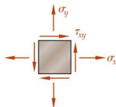
$$\sigma_x = 0 \quad \sigma_y = +56.6 \text{ MPa} \quad \tau_{xy} = +50.9 \text{ MPa}$$
