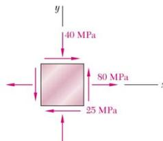
The state of plane stress shown occurs at a critical point of a steel machine component, of which tensile yield strength is 250 MPa. Determine the factor of safety with respect to yield, using (a) the maximum-shearing-stress criterion, and (b) the maximum-distortion-energy criterion.
